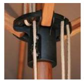
The Sirocco is designed for the commercial and domestic markets with the Bambrella® three key points of design - durability, strength and style. The main feature of the Sirocco is the use of nylon for the hub and runner, which have built in rollers for the rope pulley system and a patented locking cleat. This clamps the rope so there is no need for the use of a pin to hold the canopy up.
