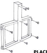
Screw the plastic feet (**F**) to the underside of the base frame (**A**).
