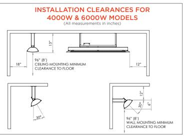
\*Alternatively, short mounting brackets can be used for wall mounting of the 4000w & 6000w models to position the heater closer to the wall. Short mounting brackets must be purchased separately.
