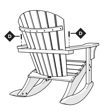
Push back up to seat-No pilot holes for final screws
